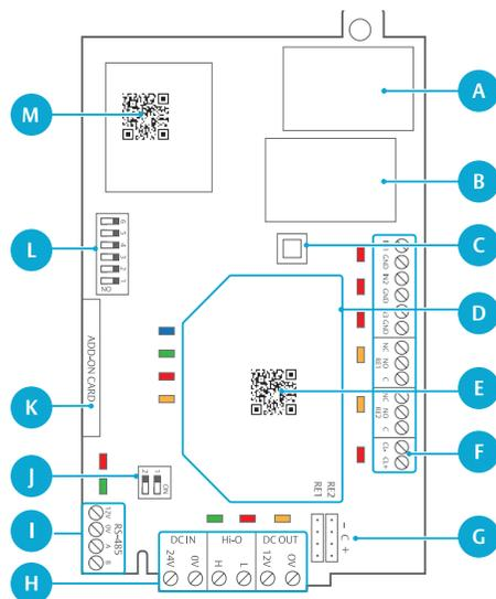
Controllers are equipped with an additional controller board (D), but the I/O connectivity is the same for both controller units.
