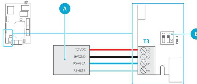
External RS-485 reader or bus (A), termination DIP (B).
