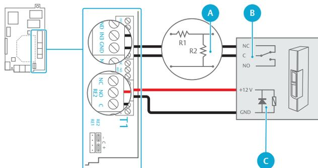
Optional dual loop (A), door sensor (B), flyback diode (C).
