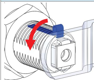
With the turn limiter assembled in upper position the catch can only be turned 90 degrees counter clockwise.
