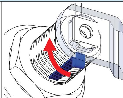
With the turn limiter assembled in lower position the catch can only be turned 90 degrees clockwise.
